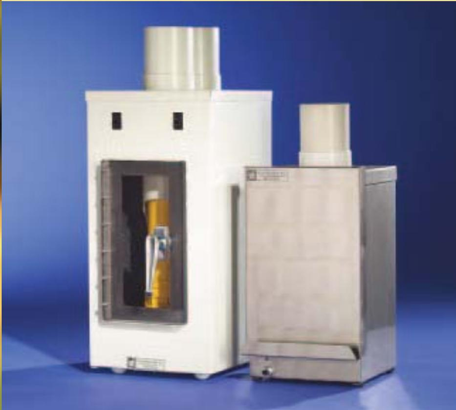
The Eagle Pneumatic Ticket Delivery System transports tickets 25 per second up to 1,000 feet through a single, connecting tube between the truck scale and the batchman/dispatch office. It can save between 3 and 5 hours of truck time for each 100 trucks that move through your yard.
